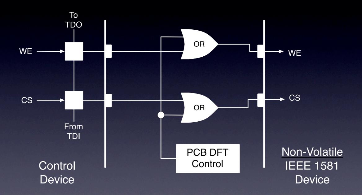
Test mode is entered if a predetermined set of logical input states exist at a predetermined period after device power-up.
